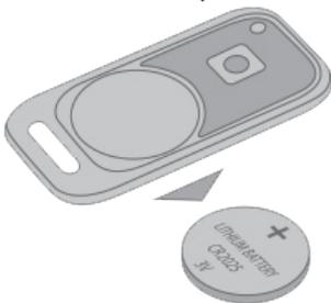
2. Press and hold the tag button and insert the power element. The LED of the tag will light up red.
