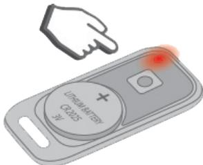
4. Successful registration will be confirmed by a green flash, 2 flashes of the LED on the transceiver, and 2 sound signals. If the tag is not registered, the LED of the tag will remain red.
