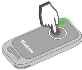
After the LED stops flashing, there will be a short green flash, after that the LED will turn red.
