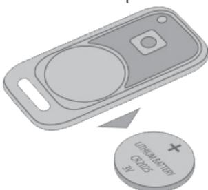
2. Insert the power source into the tag.
