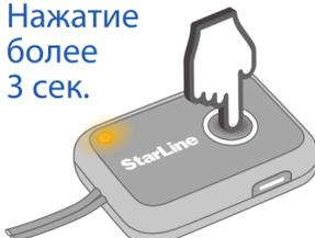
4. Release the button. There will be 5 short signals with the green LED flashing.
