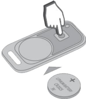
3. Keep the tag button pressed for at least three seconds, then release it.
