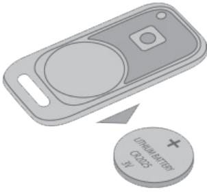
2. Press and hold the button on the tag, then insert the battery back into the tag.
