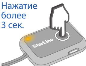
7. Release the button. Seven short beeps will follow, with the green LED flashing. The immobilizer will enter "Device Registration" mode.
