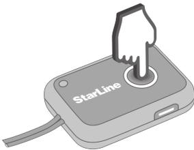
3. Yellow flashes will follow, accompanied by sound signals. Count the number of flashes equal to the first digit of the unlock code and briefly press the indicator module button. The entry of the first digit is complete.
