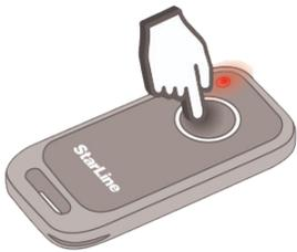
4. Successful setting of the low sensitivity level for the motion sensor will be confirmed by three beeps.
