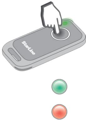
3. Press the tag button 3 times while the LED is red. After the red LED stops flashing, there will be a series of red flashes corresponding to the number of presses.
