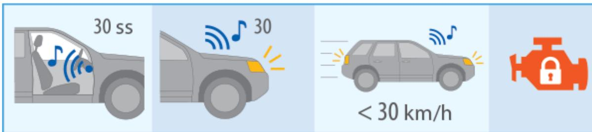
Exit from the «Anti hijack» mode and engine unblocking is performed by one of the following methods:
