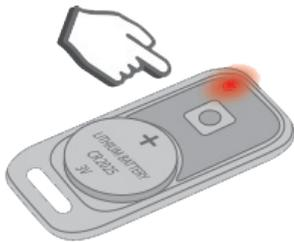
4. Successful registration will be confirmed by a green flash and 2 LED signals. If the tag was not registered, the LED will light up red.
